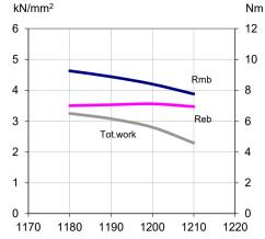
Hardening Temperature in °C Original dimension Ø 5.6 mm Tempering 4 x 1 hour at 560°C Dimension of test piece Ø 4.7 mm
