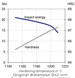
Tempering 4 x 1 hour at 560° C Unnotched test piece 7 x 10 x 55 mm
