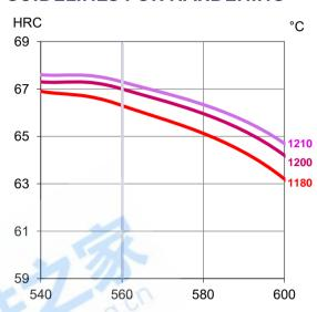
Tempering Temperature °C Hardness after hardening, quenching and tempering 4x1 hour
