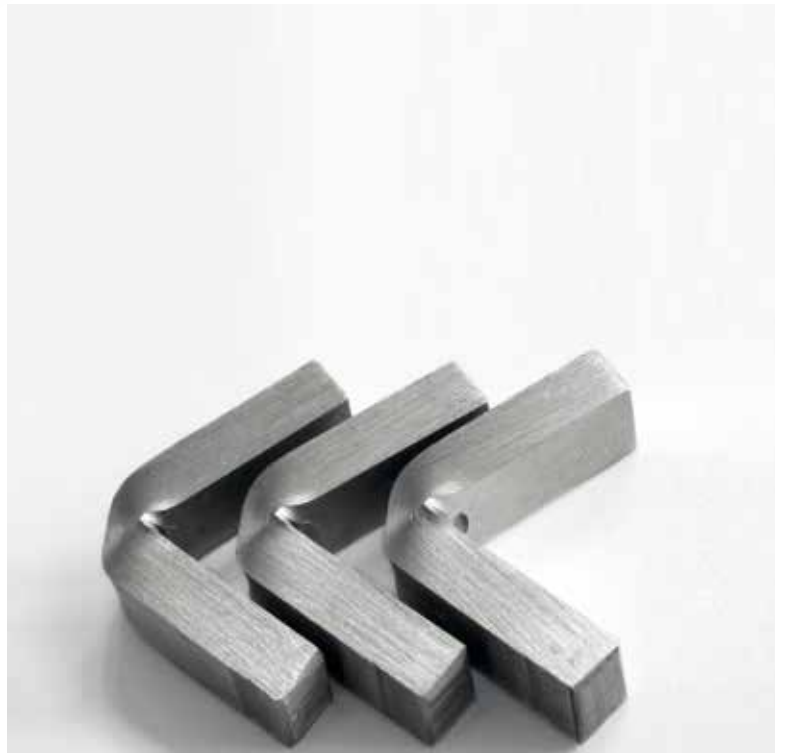
Impact bending samples (tempered to 44 - 46 HRC) after testing on a 450J pendulum impact testing machine
