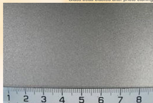
● 微細梨地シボ加工例 Example of precise creping
