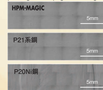
↑ 溶接ビードの境界部 The border line of the welding bead
